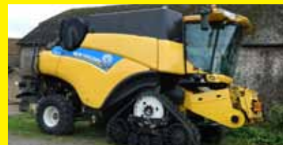
New Holland CR8080 with 24" tracks Varifeed 30 foot high capacity header, 2 x side knives, tandem axle trolley.
